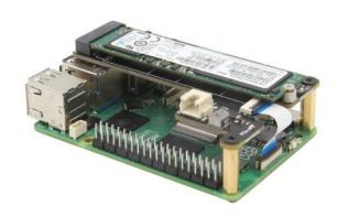
X1001 V1.1 NVME M2 SSD Shield for Raspberry Pi 5
